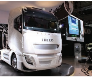
Above: Iveco's futuristic Glider concept tractor features several fuel-saving devices, such as 'smart cooling', waste heat recovery and a belt-less engine
